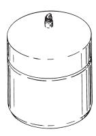
INSTALL THERMAL EXPANSION TANK OR DEVICE IF WATER HEATER IS INSTALLED IN A CLOSED WATER SYSTEM.
